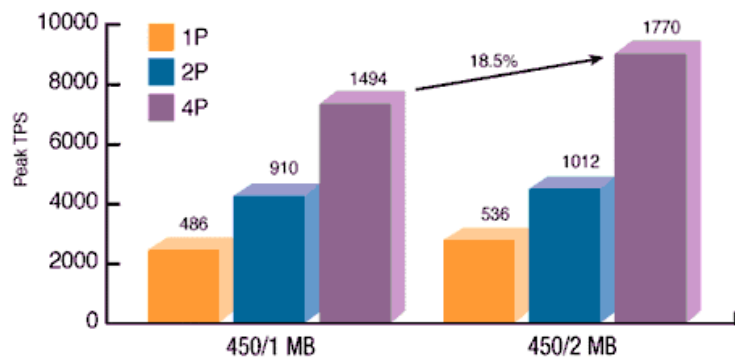
FIGURE 7. MULTIPROCESSING BENCHMARK RESULTS PUBLISHED BY INTEL IN 1998. LOOK CAREFULLY — THE RESULTS DEPICT MEASUREMENTS OF 1, 2 AND 4-WAY SYSTEMS, COMPARING SIMILARLY CONFIGURED SYSTEMS WITH 1 AND 2 MB OF LEVEL 2 CACHE.
